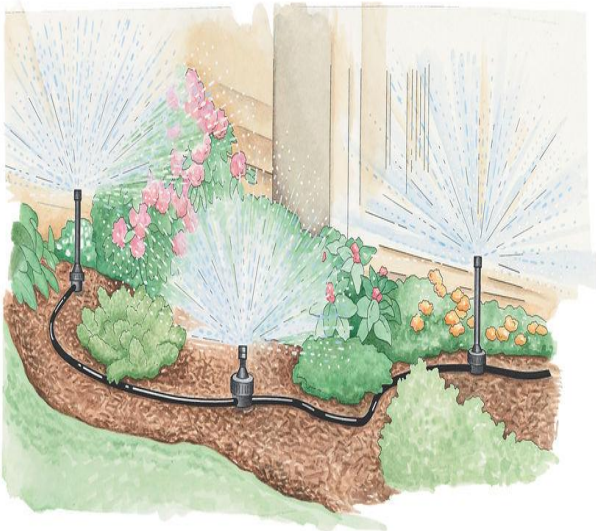
Soakers with Risers/Sprinkler heads
